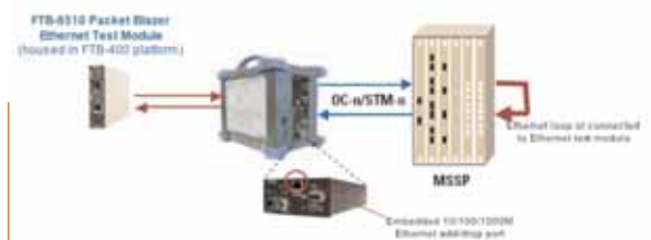
The FTB-8120NG/8130NG module's embedded 10/100/1000M Ethernet and Gigabit Ethernet interfaces allow users to extract and insert Ethernet payload to/from a GFP-mapped OC-n/STM-n line, providing a powerful test solution for Ethernet-over-SONET/SDH service validation.
