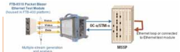
Combining the FTB-8510's Ethernet multiple-streaming capabilities and the FTB-8120NG/8130NG embedded Ethernet interfaces creates a powerful solution for testing multiple services over SONET/SDH.
